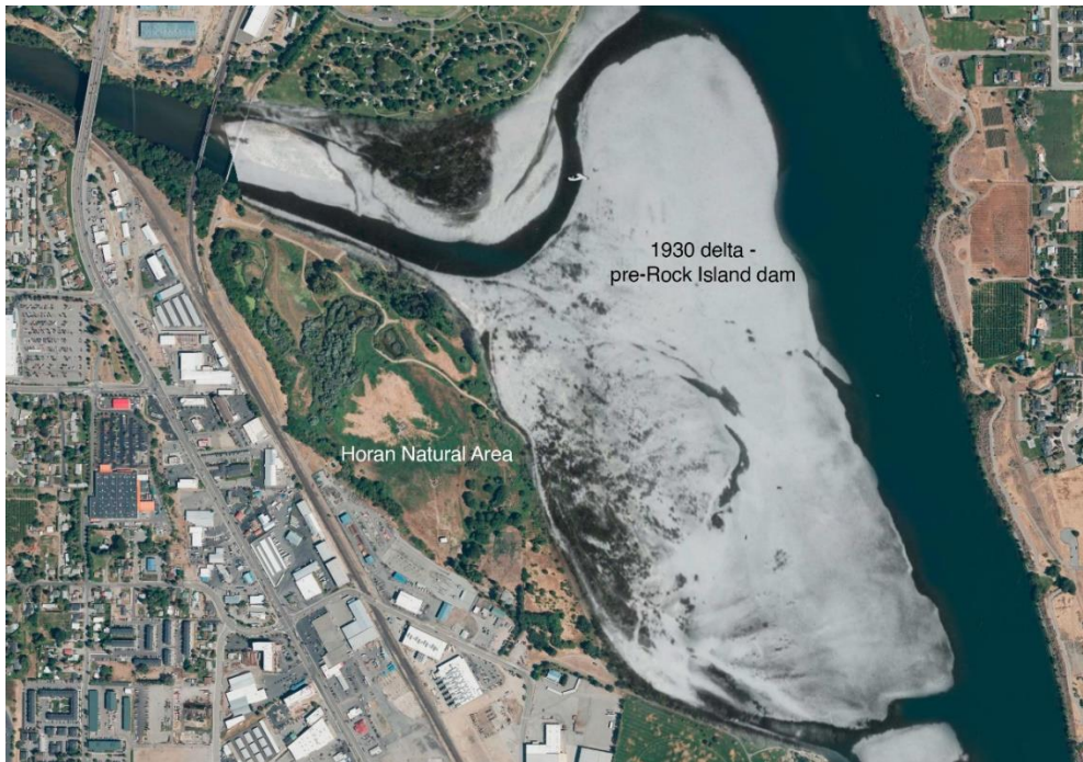
Figure 2. The Horan Natural Area (color) and the historic extent of the Wenatchee River delta that is currently inundated by the Rock Island dam operating pool (gray, 1930)
